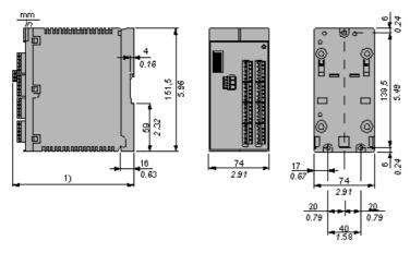
(1) 153 mm (6.02 in) with XPSMCTS• 151.4 mm (5.96 in) with XPSMCTC•
