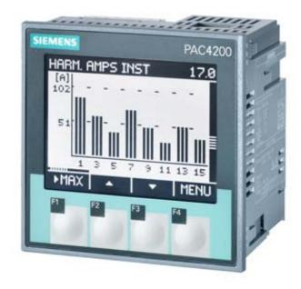
SENTRON PAC4200, LCD, 96X96MM POWER MONITORING DEVICE PANEL MOUNT TYPE FOR MEASUREMENT OF ELECTR. VALUES VAUX: 22-65VDC VIN: MAX.500/289V, 45-65HZ AMPIN: X/1A OR X/5A AC COMPRESSION TYPE TERMINALS
