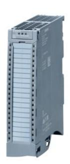
SIMATIC S7-1500, ANALOG INPUT MODULE AI 8 X U/I HF, 16 BITS OF RESOLUTION, ACCURACY 0.1%, 8 CHANNELS IN GROUPS OF 1; COMMON MODE VOLTAGE: 30V AC/60V DC, DIAGNOSIS, PROCESSALARMS; INCL. INFEED ELEMENT, SHIELD CLAMP AND SHIELD TERMINAL
