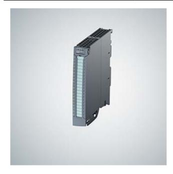
SIMATIC S7-1500, DIGITAL OUTPUT MODULE DQ 16 X 24VDC/0.5A; 16 CHANNELS IN GROUPS OF 8, 4 A PER GROUP; DIAGNOSIS; SUBSTITUTE VALUE
