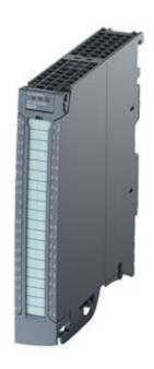
SIMATIC S7-1500, DIGITAL INPUT MODULE, DI32 X DC24V, 32 CHANNELS IN GROUPS OF 16; INPUT DELAY TYP. 3.2MS; INPUT TYPE 3 (IEC 61131) INCL. FRONT CONNECTOR PUSH-IN
