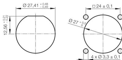
Mounting cut-out: 1. With central screw connection / 2. For mounting with four M3 screws
