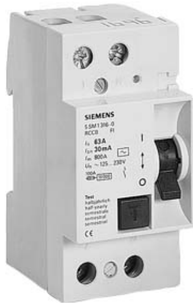
RES.CURRENT OP.CIRCUIT BREAKER TYPE AC WS D=55MM 63A 1+N-POL IFN 30MA 230V 2,5MW
