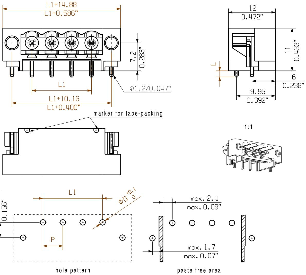
For the mounting of PCBs, it should be noted that the rated data given in the catalogue relates only to the connection elements. The necessary creepage and clearance paths must be observed in connection with the respective applicant in accordance to VDE 0110. The current-carrying capacity and pitch tolerance is to be determined according to DIN IEC 326 part 3 very fine.
