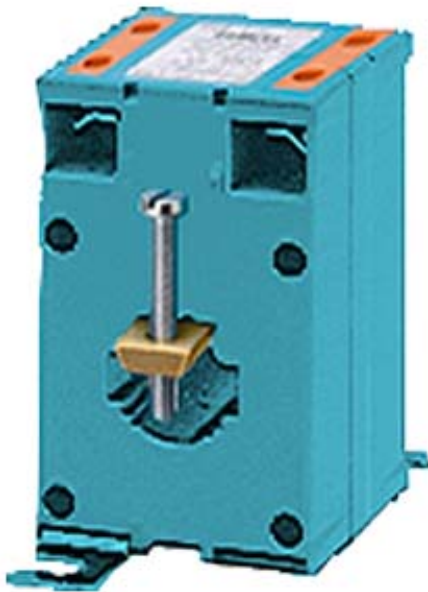
WINDOW-TYPE CURRENT TRANSFORMER, CLASS 1 200A/5A, 5VA PRIMARY CURRENT 200A, 5VA
