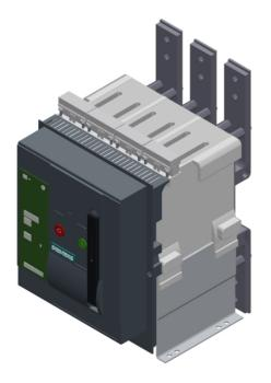
FIXED-MOUNTED CIRCUIT BREAKER 3-POLE, SIZE I, IEC IN=1250A TO 690V, AC50/60HZ ICU=55KA AT 500V FRNT.CONN. TOP/BOT. DUAL-HOLE ELECTRONIC TRIP UNIT ETU 15 LI PROT. ADJUST.B. 0.5-1 IN MOT./MAN. OPER.MECHAN. W.STOR. DRIVE MOTOR AC 50/60HZ 208-240V BZW DC 220-250V REQU. AC 50/60HZ 230V, DC 220V WITHOUT 1ST SHUNT TRIP WITH 2ND AUX. RELEASE "R", F3 UNDERVOLTAGE, NON-DEL. AC 208-240V, DC 220-250V 2NO+2NC
