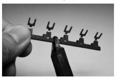
When using a cut short-circuit bar (P2DN), always use the provided cap to protect the charger part.
