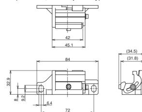
Material: Zinc alloy, Fluorochemical lubricant oil
