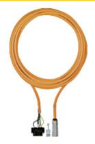
Cable for PMCprotego and motor with connector design assembled on both sides with connector <> round connector 8-pin No. of wires and cross section  $(4 \times 4 + (2 \times 1,5))$  Trailing, length: 10 m.
