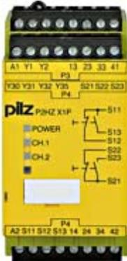
Safety relay (standalone) Inputs: 1 N/O, 1 N/C per pushbutton Outputs: 3 N/O, 1 N/C, 2 semiconductor UB 24 V AC, width: 45 mm, plug-in terminals of screw type Two-hand control device/monitoring the simultaneity of two-hand pushbuttons.
