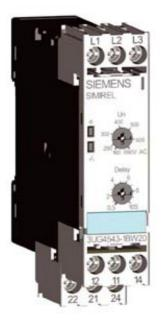
DC AND AC 50 TO 60 HZ 2-POINT OR 1-POINT CONTROL TRIPPING DELAYED 0.5 TO 10S 1 CHANGEOVER CONTACT SPRING-LOADED TYPE
