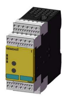
SIRIUS SAFETY RELAY FOR SAFETY-ORIENTED STANDSTILL MONITORING, 400V AC, 45.0MM, SPRING-LOADED TERMINAL, FK INSTANT.: 3NO 1NC, FK DELAYED: 0, MK: 3, AUTO START, BASIC UNIT, MAX. ACHIEV. CAT. EN954-1: 4,
