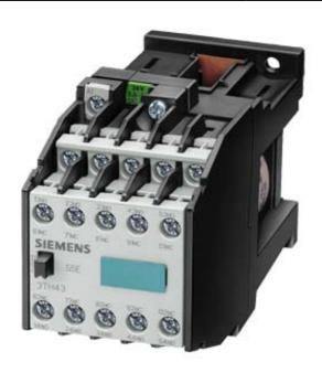
CONTACTOR RELAY 54 EN 50 011 5NO+4NC F.SNAP-ON AND SCREW MOUNTING WITH MECHANICAL LATCHING DC OPERATION DC SOLENOID SYSTEM DC 220V
