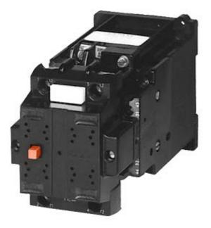
CONTACTOR SIZE 2 2-POLE WITH DELAYED DISCONNECTION. AUX. SWITCHES 2NO + 1NC 380/440 V AC 50 HZ/60 HZ
