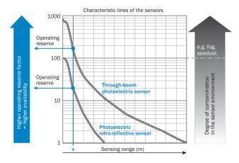
At a sensing range of  $\tt ,x''$  the photoelectric retro-reflective and through-beam photoelectric sensors have different operating reserves (see blue arrow). The higher the operating reserve factor, the better the sensor can compensate the contamination in the air or in the light beam and on the optical surfaces (front screen, reflector), i.e. the sensor has the maximum availablity, otherwise the sensor switches due to pollution although there is no object in the path of the light beam.
