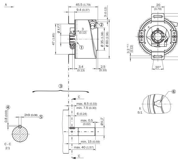
① Operating temperature measuring point (freely selectable, around the housing surface area in each case, approx. 3 mm away from flange)
