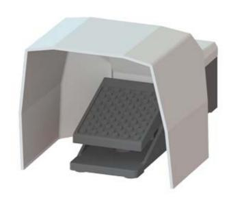
FOOT-OPERATED BUTTON, SINGEL PEDAL (WITHOUT LATCHING) CABLE ENTRY M20X1,5 IP 65, 2NO + 2NC WITH COVER
