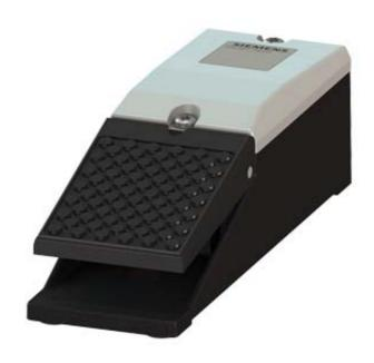
FOOT -OPERATED BUTTON, SINGLE PEDA L(WITHOUT LATCHING), CABLE ENTRY 1X(M20X1,5) METAL CASING IP65, 1 NO + 1 NC WITHOUT PROTECTIVE COVER
