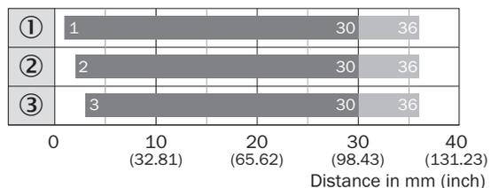
■ Sensing range      ■ Sensing range max. typ.
