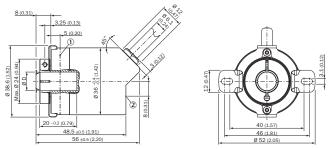
Non-tolerated dimensions according to DIN-ISO 2768-mk
