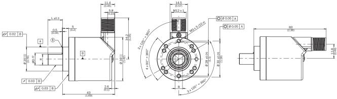
① Measuring point for operating temperature
