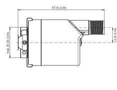
① Measuring point for operating temperature
