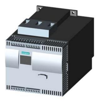
SIRIUS SOFT STARTER, VALUES WITH 500 V, 40 DEG., STANDARD: 29A, 18,5KW, INSIDE-DELTA CIRCUIT 3: 50A, 30KW, 400-600 V AC, 230 V AC, SCREW TERMINALS
