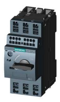
CIRCUIT-BREAKER SZ S00, FOR MOTOR PROTECTION, CLASS 10, A-REL. 0.14...0.2A, N-RELEASE2.6A, SPRING-L. CONNECTION STANDARD SW. CAPACITY W. TRANSVERSE AUX. SWITCH 1NO+1NC
