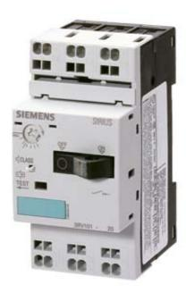
CIRCUIT-BREAKER, 7...10 A N-RELEASE 130 A, SIZE S00 MOTOR PROTECTION, CLASS 10, CAGE CLAMP CONNECTION STANDARD BREAKING CAPACITY
