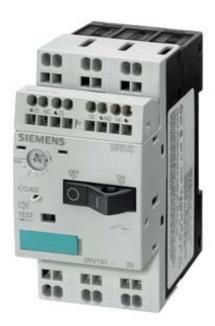
CIRCUIT-BREAKER, SIZE S00, FOR MOTOR PROTECTION, CLASS 10, A-RELEASE 3.5...5 A, N-RELEASE 65 A, CAGE-CLAMP CONNECTION STANDARD SWITCHING CAPACITY W. TRANSV. AUX. SWITCH 1NO+1NC
