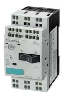
CIRCUIT-BREAKER, SIZE S00, FOR MOTOR PROTECTION, CLASS 10, A-RELEASE 0.22...0.32 A, N-RELEASE 4.2 A, CAGE-CLAMP CONNECTION STANDARD SWITCHING CAPACITY W. TRANSV. AUX. SWITCH 1NO+1NC
