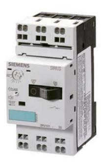
CIRCUIT-BREAKER, 0.14...0.2 A N-RELEASE 2.6 A, SIZE S00 MOTOR PROTECTION, CLASS 10, CAGE CLAMP CONNECTION STANDARD BREAKING CAPACITY
