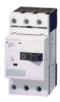
CIRCUIT-BREAKER SIZE S00, FOR MOTOR PROTECTION, CLASS 10, A-REL.0.14...0.2A,N-REL.2.6A, SCREW TERMINAL, STANDARD SWITCHING CAPACITY
