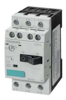
CIRCUIT-BREAKER, SIZE S00, FOR MOTOR PROTECTION, CLASS 10, A REL.0.11...0.16A, N REL.2.1A SCREW CONNECTION, STANDARD BREAKING CAPACITY, W. TRANSV. AUX. SWITCH 1NO/1NC
