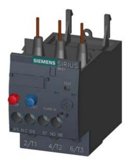
OVERLOAD RELAY 2.2...3.2 A FOR MOTOR PROTECTION SZ S0, CLASS 10, F. MOUNTING ONTO CONTACTOR MAIN CIRCUIT: SCREW TERMINAL AUX. CIRCUIT: SCREW TERMINAL MANUAL-AUTOMATIC-RESET
