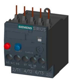
OVERLOAD RELAY 2.8...4.0 A FOR MOTOR PROTECTION SZ S00, CLASS 10, F. MOUNTING ONTO CONTACTOR MAIN CIRCUIT: SCREW TERMINAL AUX. CIRCUIT: SCREW TERMINAL MANUAL-AUTOMATIC-RESET
