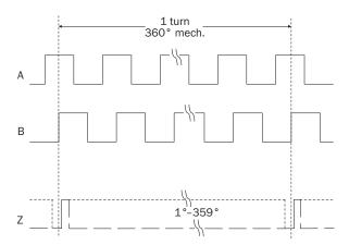
Electrical zero pulse width can be configured to 90°, 180°, or 270°. Width of the zero pulse in relation to a pulse period.
