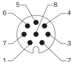
View of M23 male device connector on encoder
