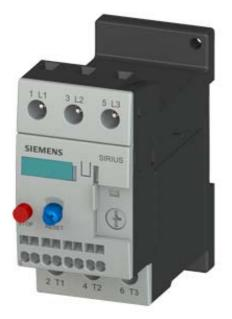
OVERLOAD RELAY, 9...12,5 A 1NO+1NC, SIZE S0, MAIN CUR.: SCREW CONNECTION AUX. CUR..: CAGE CLAMP FOR INDIVIDUAL INSTALLATION
