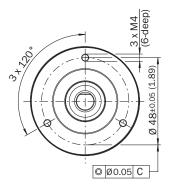
General tolerances according to DIN ISO 2768-mk ① Cable diameter = 5.6 mm +/- 0.2 mm bend radius = 30 mm
