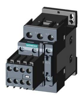
CONTACTOR, AC-3, 18.5KW/400V, 2NO+2NC, AC 110V 50HZ, 3-POLE, SZ SO SCREW TERMINAL REMOVABLE AUX. SWITCH
