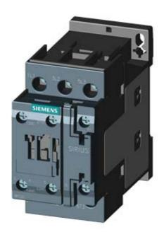
CONTACTOR, AC-3, 18.5KW/400V, 1NO+1NC, AC 110V 50HZ, 3-POLE, SZ SO SCREW TERMINAL
