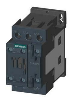
CONTACTOR, AC-3, 11KW/400V, 1NO+1NC, AC 24V 50/60HZ, 3-POLE, SZ SO SCREW TERMINAL
