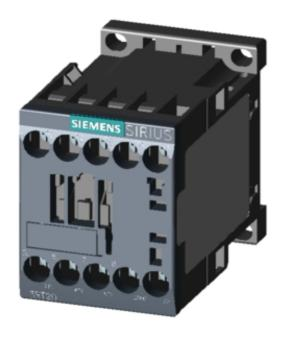
CONTACTOR, AC-3, 5.5KW/400V, 1NC, AC 48V, 50/60 HZ, 3-POLE, SZ S00 SCREW TERMINAL
