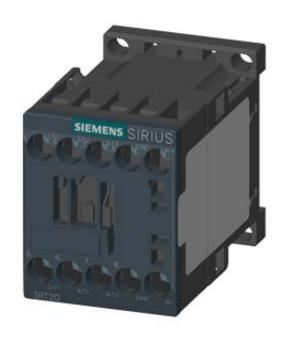
CONTACTOR, AC-3, 3KW/400V, 1NC, DC 72V, 3-POLE, SZ S00 SCREW TERMINAL
