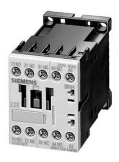
CONTACTOR, AC-3 4 KW/400 V, AC-1 18 A, CC 48 V 50/60 HZ, 4-POLE, 2 NO + 2 NC, SIZE S00, SCREW CONNECTION
