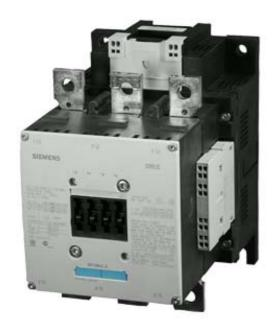
CONTACTOR, 160KW/400V/AC-3 AC(40...60HZ)/DC OPERATION UC 23-26V AUXILIARY CONTACTS 2NO+2NC 3-POLE, SIZE S10 BAR CONNECTIONS CONVENT. OPERATING MECHANISM CAGE CLAMP TERMINAL
