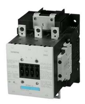
CONTACTOR, 75KW/400V/AC-3, AC(40...60HZ)/DC OPERATION UC 42...48V AUXIL. CONTACTS 2NO+2NC 3-POLE, SIZE S6 BAR CONNECTIONS CONVENTIONAL OPERATING MECHAN. SCREW TERMINAL
