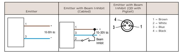
Cabled emitters with beam inhibit use the white wire to error-proof wiring in the cabinet. QD models use the standard pinout and the beam inhibit (pin 4) wire color is determined by the cordset used, but is typically black.
