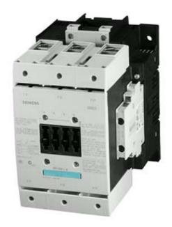
CONTACTOR, 55KW/400V/AC-3, AC(40...60HZ)/DC OPERATION UC 380...420V AUX. CONTACTS 2NO+2NC, 3-POLE, SIZE S6 WITH BOX TERMINALS CONVENTIONAL OPERATING MECHAN. SCREW TERMINAL
